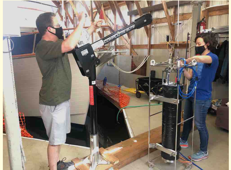
Brian Bill (left) and Alexis Fischer (right) secure IFCB to the winch line before lowering it underwater at Budd Inlet. Credit: Vera Trainer.
