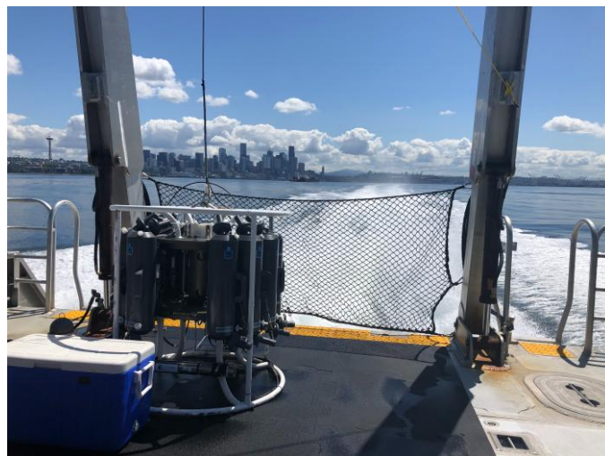
CTD profiler and Niskin bottles.
