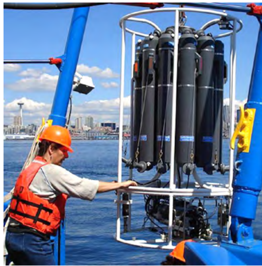
A CTD rosette collects and measure ocean water properties at different depths. Photo: UW
